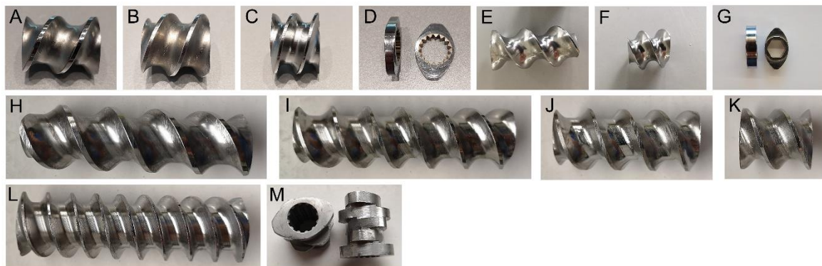
Figure 12. Screw elements used for screw configurational setup: A)-D) on the QbCon®1 and the QbCon®25, E)-G) on Pharma 16 and H)-M) on Leistritz Micro 27 GL-28D.
