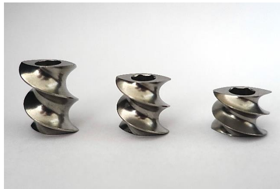
Figure 2. Exemplary photograph of conveying elements with different pitches.
