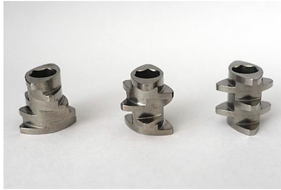
Figure 3. Exemplary photograph of kneading blocks at various offset angles.
