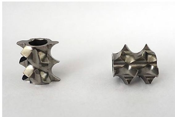
Figure 4. Exemplary photograph of distributive feed screw (kindly provided by K. Kiricenکو).
